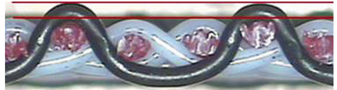
Fig. 6b: Uneven surface of a sieve with competitive material – Product side: antistatic PA & PET at different levels; machine side: the antistatic monofilament has an arched float
