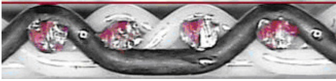
Fig. 6a: Even surface of a sieve with AntiStat – Product side: AntiStat and PET at the same level; machine side: AntiStat offers a flat and stable float
