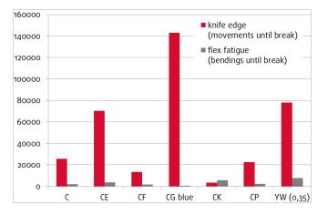
The abrasion resistance is improved by means of additives which permanently anchor additional slip properties in the polymer and simultaneously optimise the molecular crosslinking.
