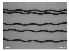
**Short Wave Filaments** Amplitude: 0.055 - 0.117 mm Wavelength: 1.80 - 2.15 mm
