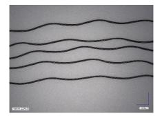
**Long Wave Filaments**Amplitude: 0.10 – 0.25 mm
