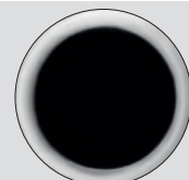
Fig. 1 Bi-component monofilament with core-sheath structure
