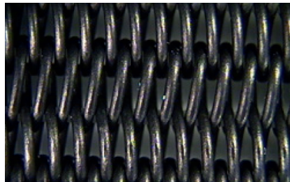
Fig. 5: Spiral fabrics from 100% AntiStat
